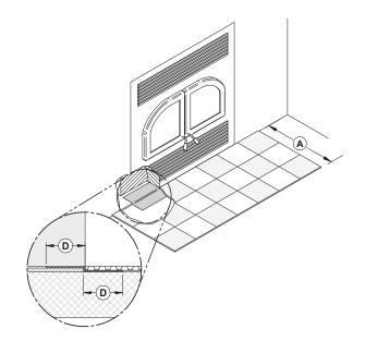
When the fireplace is installed directly on the floor, a non-combustible floor protection of at least 16" **(A)** with an R factor of 1.00 must be installed in front of the fireplace.
