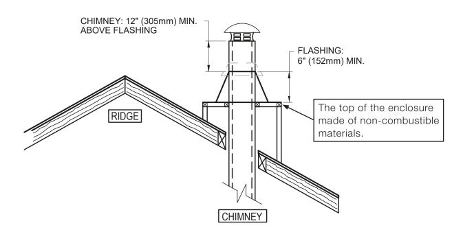
WARNING: IF THE CHIMNEY IS INSTALLED IN AN ENCLOSURE ABOVE THE ROOF, IT MUST EXCEED THE TOP OF THE FLASHING CONE BY AT LEAST 12 INCHES (30 CM). THE FLASHING MUST HAVE A MINIMUM HEIGHT OF 6 INCHES (15.25CM). THE TOP OF THE ENCLOSURE MUST BE MADE OF NON-COMBUSTIBLE MATERIALS.
