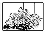
Raking the coals is useful for two reasons. First, it brings them near where most of the combustion air enters the firebox. This will ignite the new load quickly. Secondly, the charcoal will not be smothered by the new load of wood. When the embers are simply spread inside the combustion chamber, the new load smoulder for a long time before igniting.
