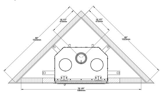
Framing configuration should be used as a reference only. If a finishing material is installed inside the enclosure, its thickness must be added to the following measurements.
