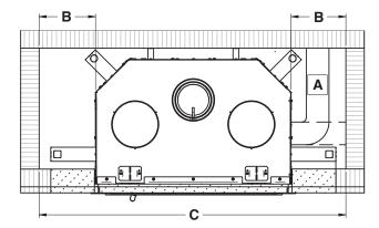
If a finishing material is installed inside the enclosure, its thickness must be added to the following measurements.
