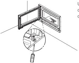
Using a flat screwdriver, turn the adjustable hinge rods in the directions shown to adjust the doors. Tighten the set screws on the door hinges when they are in the desired positions.
