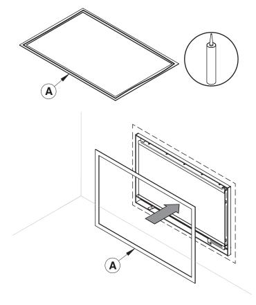
Secure the finishing frame to the facing using silicone.
