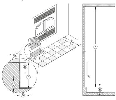
When the fireplace is installed on a raised base of more than 4" (E), a non-combustible floor protection of at least 16" (A) with no R factor must be installed in front of the fireplace.
