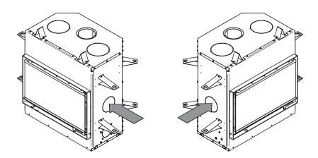
This kit allows distributing heat to another room up to 50 feet (15 m) of the fireplace. The insulated flexible pipe (not included in the kit) must be HVAC type pipe and must comply with ULC S110 and/or UL 181, Class 0 or Class 1 Standards and must withstand temperatures up to 250°F. For the complete installation procedure, see the installation manual provided with the kit.
