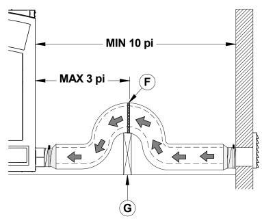
It is strongly recommended to install a mechanical shutter that closes the outside air inlet when the fireplace is not in use.
