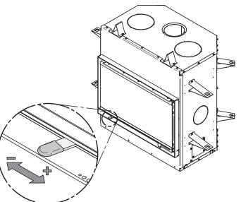
On the other hand, too much air can make the fire uncontrollable, creating very high temperatures in the unit as well as in the chimney and seriously damaging them. A reddish glow on the unit and on the chimney components indicates overheating. Excessive temperatures can cause a chimney fire.
