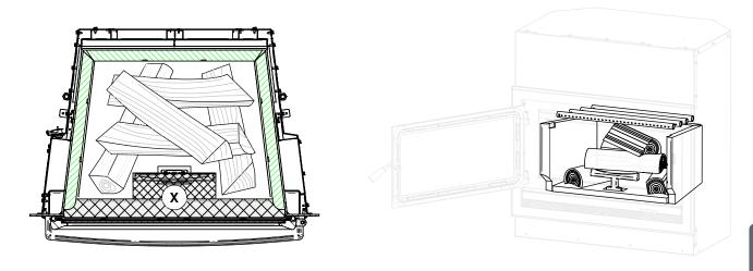
The images above show the space in the firebox where the logs are to be placed. It is important to always respect this space and not to put logs in the grid area marked with an X. The marked area is defined by the space between the glass and the cast-iron andiron. To have a good ignition, place the two lower logs in a north-south position and cross the others on top. Leave enough space between the logs for good air circulation. The log length recommended for this fireplace is 16 in.
