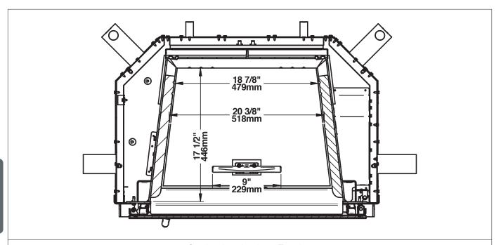
Combustion chamber - Top view
