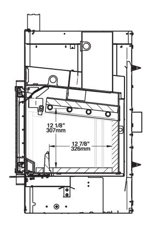
Combustion chamber - Side view
