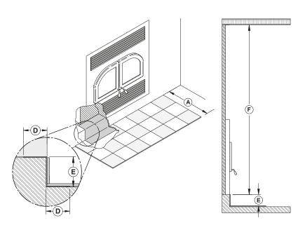
When the fireplace is installed on a raised base of 4" or less (E), a non-combustible floor protection of at least 16" (A) with an R factor of 1.00 must be installed in front of the fireplace.
