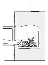
Do not leave the fireplace unattended when the door is slightly open. Always close and latch the door after the fire ignites.
