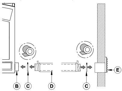
5. To complete the installation, make a hole of ¼" to ½" (6 mm to 13 mm) bigger than the duct diameter on the outside wall of the house at the chosen location. From outside, place the outside wall register in the hole (open side down) and fasten the register to the wall, with screws.
