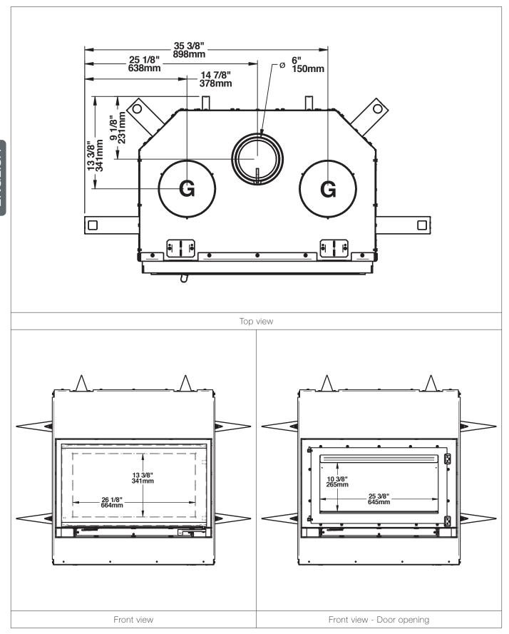
**G**: Opening for gravity hot air distribution kit (Ø 8").
