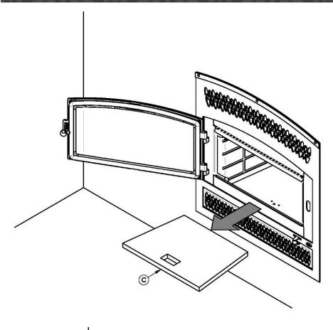
2. Remove the floor refractory slab (C).
