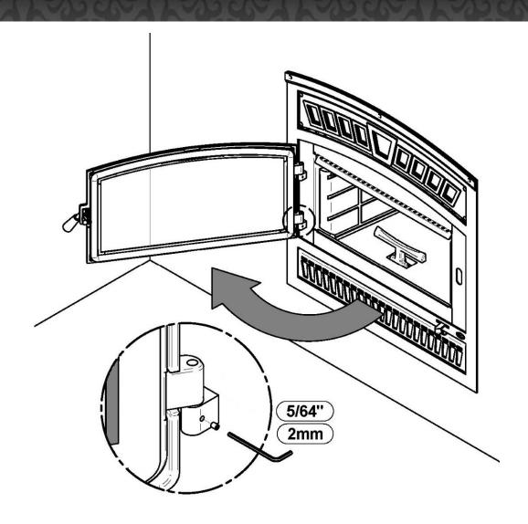
Using a flat screwdriver, turn the adjustable hinge rods in the direction shown to adjust the doors. Tighten all door hinge pressure screws when they are at the desired positions.
