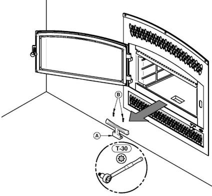
1. Using a ratchet key and a Torx (T-30), unscrew the two Torx screws (B) holding up the andiron (A).
