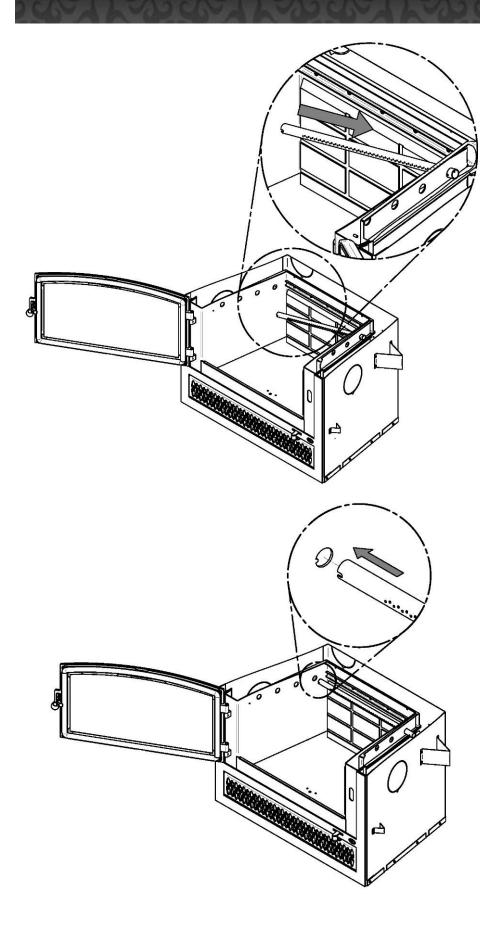
4. Starting with the rear tube, lean and insert the right end of the secondary air tube into the rear right channel hole. Then, lift and push the tube towards the right inside the hole in the right channel.
