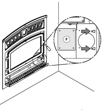
(3) Flip the fireplace's lower decorative louver. Install the blocking plate (F) included in the kit, on the front opening of the air control housing. Using a screwdriver, secure with two screws.
