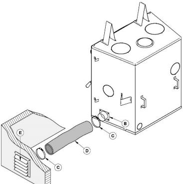
(4) Then, install the flexible pipe\* (D) (not supplied) to the fresh air intake adapter (B) using one of the adjustable pipe clamps (C). Secure the other end of the pipe to the outside wall termination (E) using the second adjustable pipe clamp (C). The outside wall termination (E) must be installed outside of the building.
