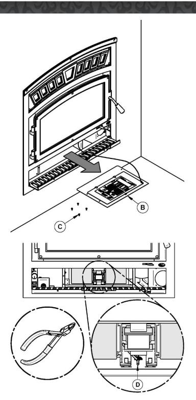
3. Remove and keep the heat shield (B) and the 4 screws (C).
