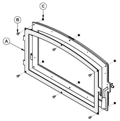
Position the overlay (A) and on the door frame and secure from the inside of the door using the 6 included screws (B) and bolts (C).
