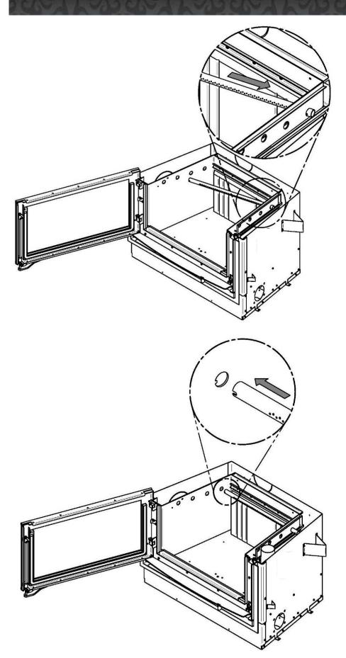
Starting with the rear tube, lean and insert the right end of the secondary air tube into the rear right channel hole. Then, lift and push the tube towards the right inside the hole in the right channel.
