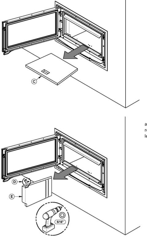
Using a power screwdriver and a 5/16" hexagonal socket, remove the slab holder (D) and the left refractory slab (E).
