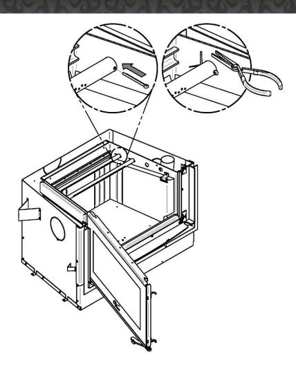
Insert a cotter pin in the last hole on the right side of the tube. Then bend the tabs on the pin to keep in place.
