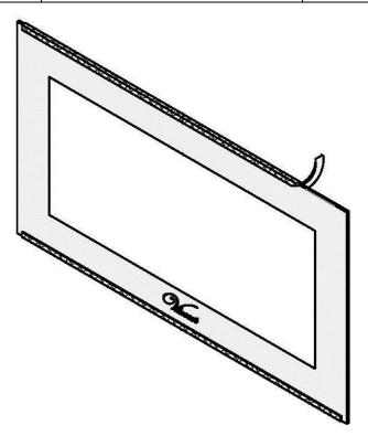
An other glass gasket is located at the back of the glass. When replace in the glass or as needed, install according to following illustrations.
