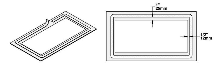
Reinstall the glass, being careful to centre the glass carefully in the door. Do not over-tighten the screws. Note that the two main causes of broken door glass are uneven placement in the door and over-tightening of retaining screws.
