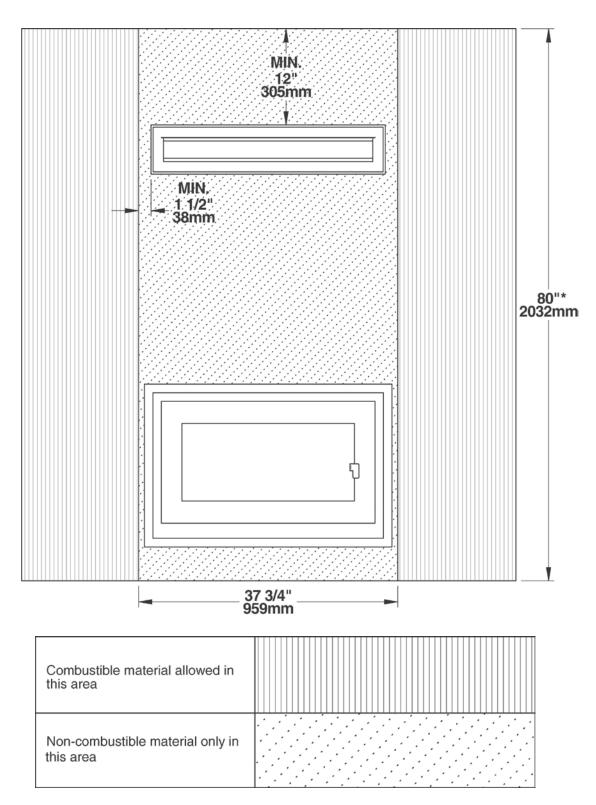
\*Must be measured from the base of the fireplace and not from the floor.
