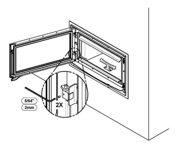
Using a flat screwdriver, turn the adjustable hinge rods in the direction shown to adjust the doors. Tighten all door hinge pressure screws when they are at the desired positions.
