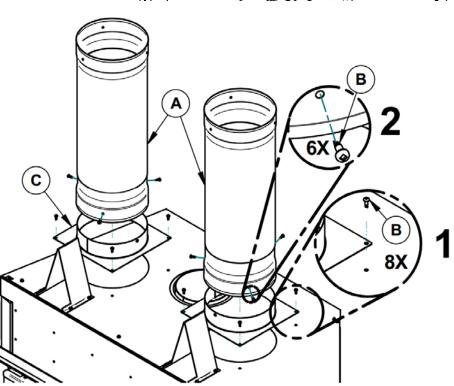
3. Secure the telescoping sections (A) to the heat distribution box (C) with self-tapping screws (B) (3 per telescoping section). Determine the needed height and secure the two parts of the telescoping sections together with 3 self-tapping screws provided. Insert the adjustable frame (D) in the heat distribution box (C), press it against the non-combustible finishing material and secure with 4 screws into the heat distribution box. Set the decorative plate (E) to the adjustable frame (D).
