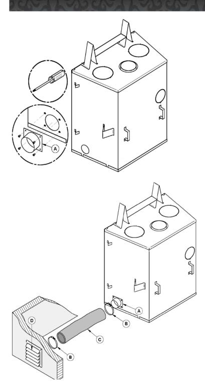
Secure the fresh air intake adapter **(A)** on the fireplace jacket using the 4 screws provided with the kit.
