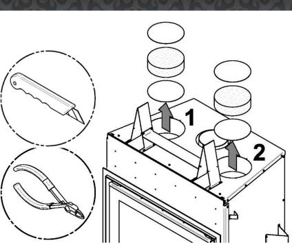
Secure the 6 steel brackets (B) with 6 screws provided (C) on top of the fireplace (3 for each ducting). Insert the ducting (A) (not provided) into each opening and secure it in place using the steel brackets (B) installed previously with 6 other self-tapping screws provided (C).
