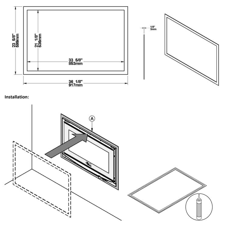
Set the finishing trim around the fireplace frame. If desired, the back of the finishing trim may be glued.
