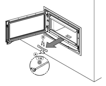
Remove the floor refractory slab (C).
